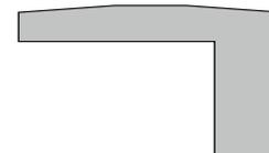
The belt thickness, the price of which is indicated in red (525), is 1.5 mm and that of the others (535) is 2 mm.
