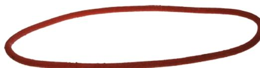
**Must be indicated:** the string length equivalent to the working tightened length. In any case it is a matter of the length of a string embracing the pulleys. Because of their elasticity, the belts are delivered in free length that is inferior from 10 to 12 % to the working length
